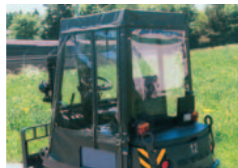
Kabine an Still-Gabelstapler.
